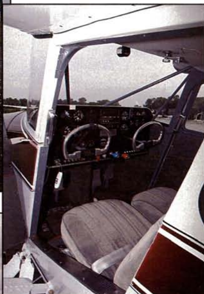
(Above) Completely re-done interior reveals a new instrument panel with all new instruments, chrome plated assist handles and trim crank on cabin roof. The rich looking seats and interior panels really caught the eye of the judges. Note the tiny float hanging on the key chain, an absolute necessity with seaplanes.
