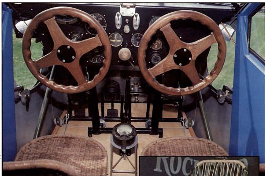
(Above) The cockpit of the Stinson is complete down to the Earth Inductor Compass installed for the flight, since a regular magnetic compass would be useless in the northern latitudes near the Arctic Circle. The caned seats were re-woven by Gar Williams (see inset) and the Pioneer instruments were in nearly working condition after 41 years on the Greenland ice cap.
