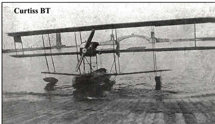
(Above) Original configuration of the Curtiss Model BT, built at the Curtiss plant in Buffalo, NY. Note the short hull, the two propellers driven by extension shafts and rotating in opposite directions, and the tail surfaces supported by booms.
