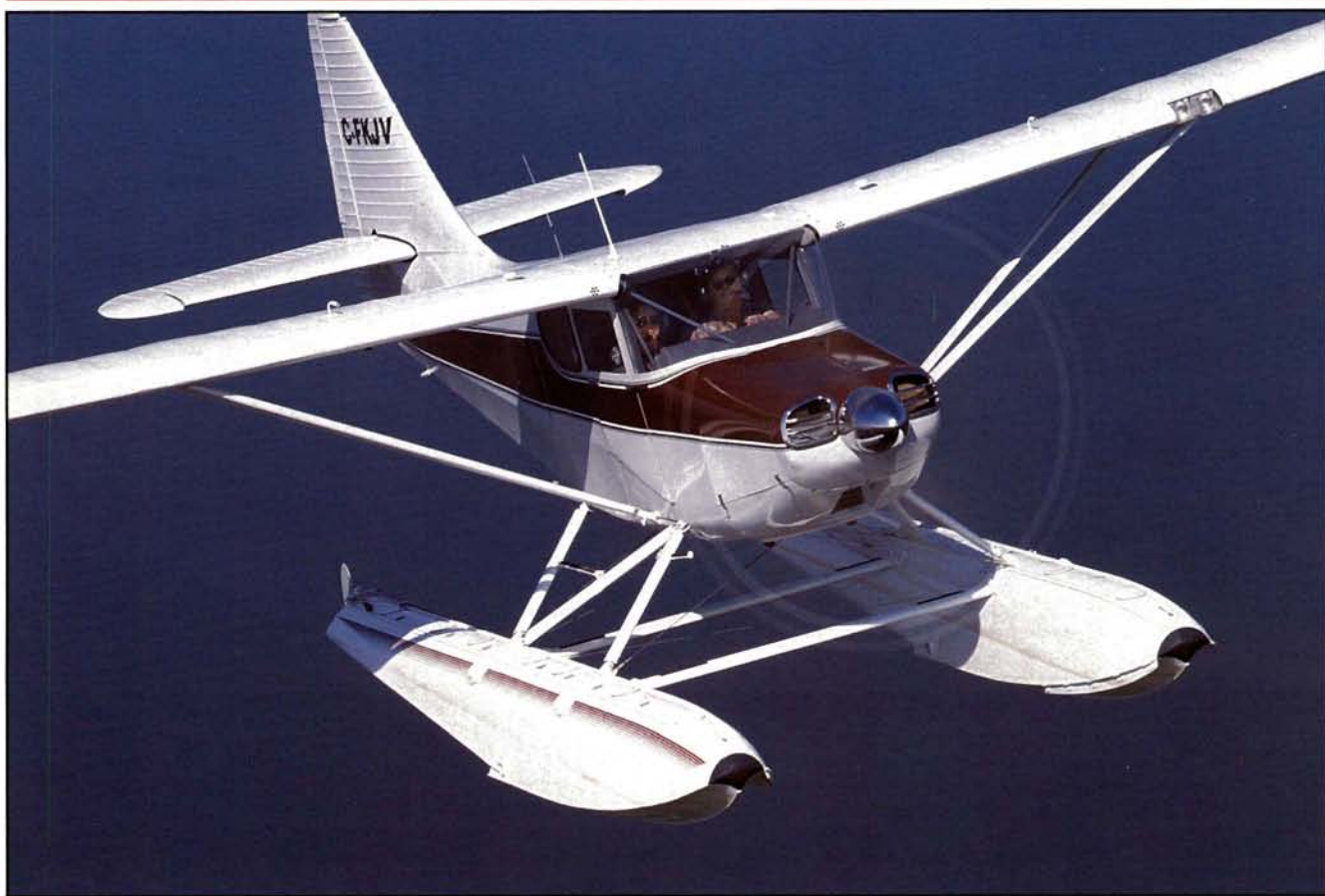
Heading right at you are Ric and Jason Henkel in the award winning Super Stinson, C-FKJV, mounted on round-topped Edo 2440 floats. The chrome plated spinner and cowl grills are visible as well as the highly polished stainless cowl fasteners. Note anti-splash rails on inside edges of the floats
